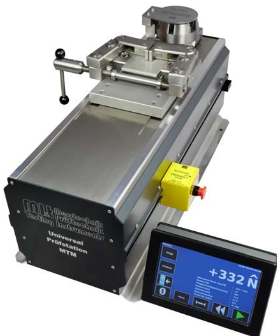
Test Station MTM 1000 with SG 90 and SHA-40W/A
