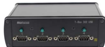
USB-Interface-Box with 4 RS232 ports
