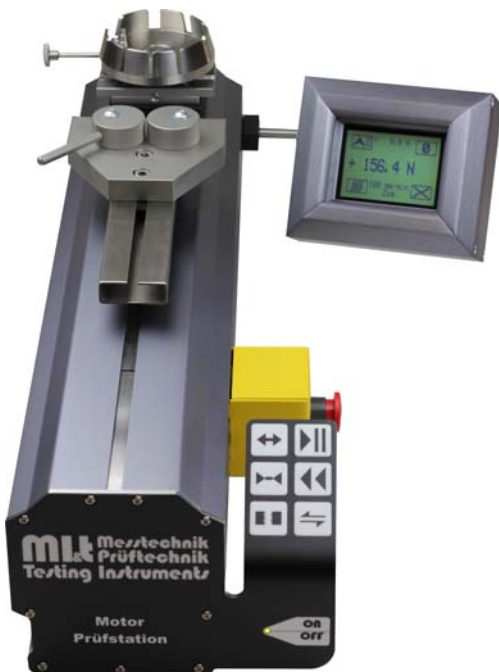
ATM 100 with tools SG 80 and DKS-20/A
