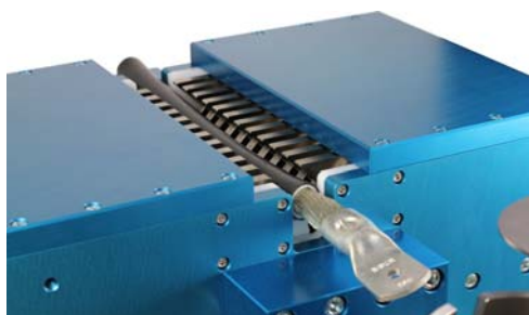
Detail: Cable clamping device with inserted cable
