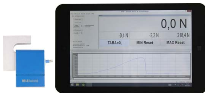
Measured valued display with force/time graph
